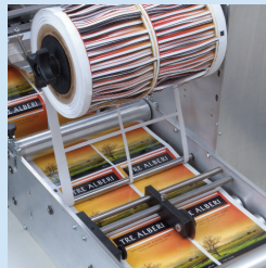
Removal of waste matrix
