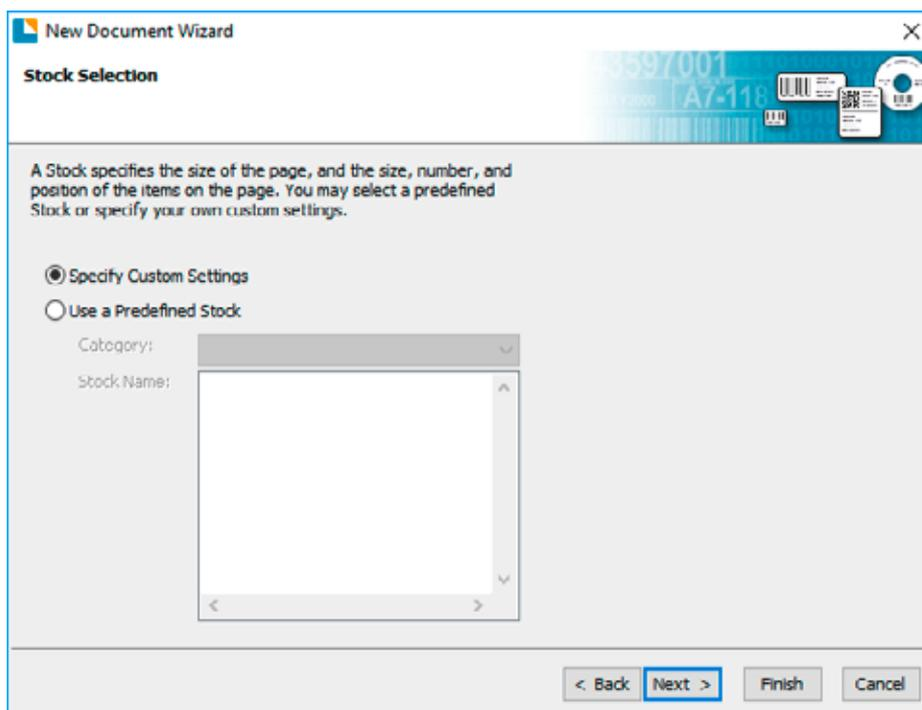
5. Set the page size, width and height to match labels installed in the printer. Click "Next". Important:
