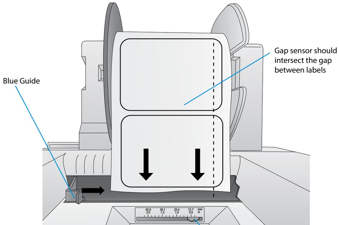
**Note:** the position of the label sensor. Slide the sensor position indicator so that it intersects with the gaps between your labels. For most label stock you will not need to move this.
