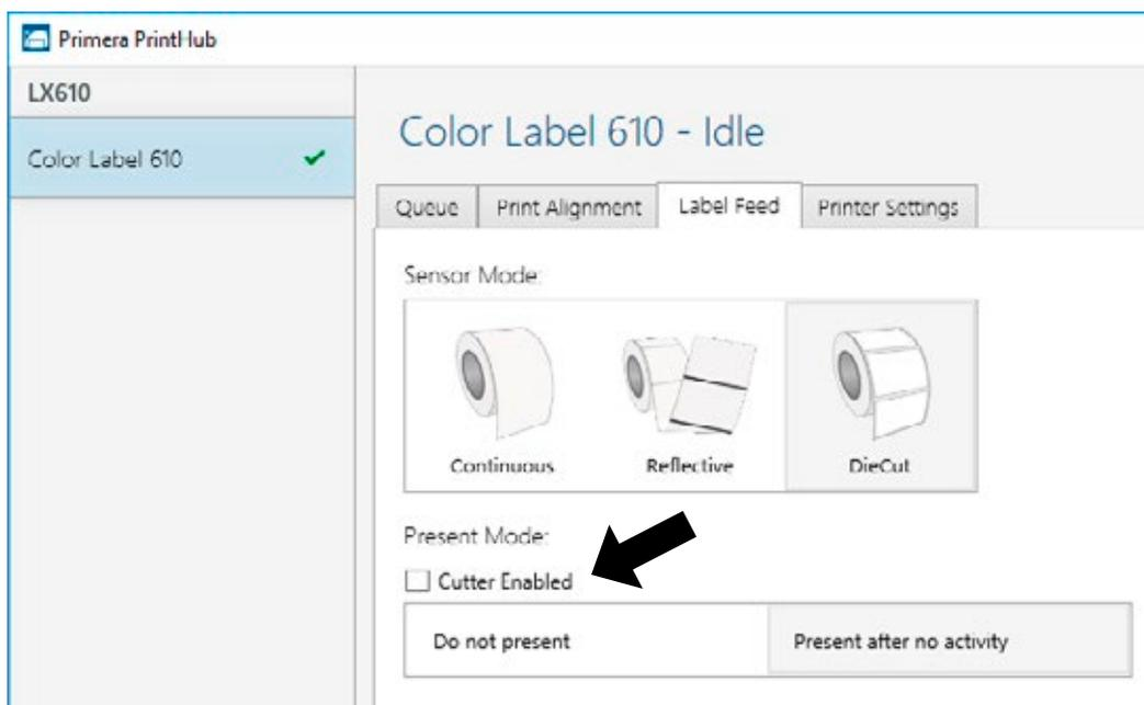
**Do not present.** In this mode the label stock does not move after the last label is printed. This means that part of the last label printed is still in the printer. This should be used only if you have a label rewinder attached.
