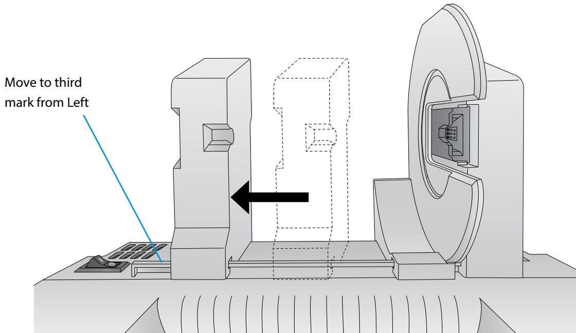
2. Install the Blue Hub on the open side of the digital die-cutting media.
