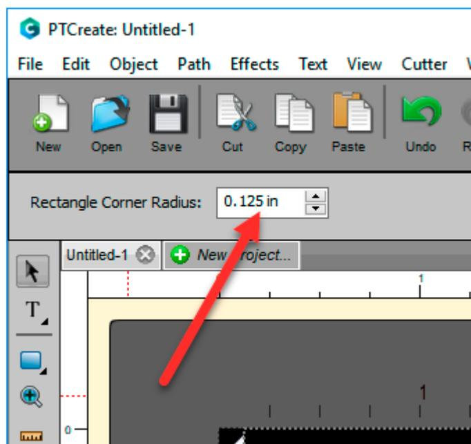
3. Draw the cut line by hovering your mouse over the top left corner of your design. When you are ready to start, left click and hold to start the rounded rectangle box. Keep holding the left mouse button and move to the lower right corner of your design. Let go of the mouse button when your box is the approximate size you would like it. We will adjust the exact size and position in the next step but to maintain a proper corner radius it is important to get as close as possible in this step.
