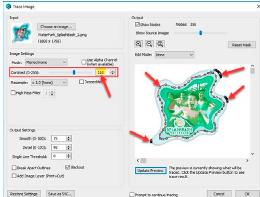
**Contrast to Low:** If contrast is too low you will end up with extra cut lines outside of the main cut and potentially the wrong shape. In this example the cut line is tracing the wrong part of the image.
