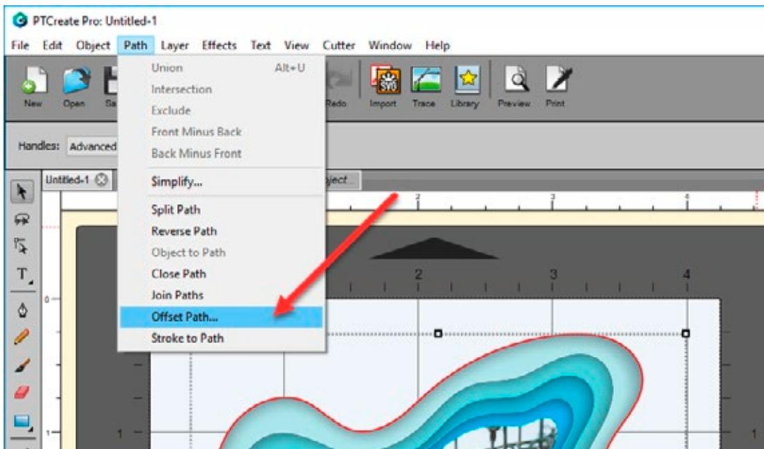
2. On the Path Offset Window, check the Inset Offset box and adjust the amount of offset. For this image we chose 0.040 inches. You'll see a preview of the new position of the cut line in black.
