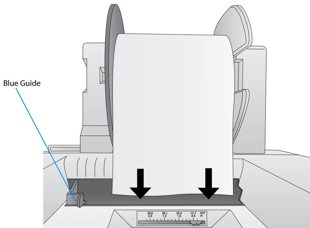
7. Push until the printer detects the stock, grabs it and pulls it through the printer.
