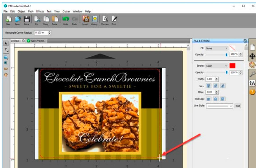
4. Once the cut line is in place you can adjust its size and position. Whatever size you choose will be the exact size of final cut label. A typical overbleed is 1/16". This will ensure that the cut is completely within the printed label every time so you have no white space around the edges.
