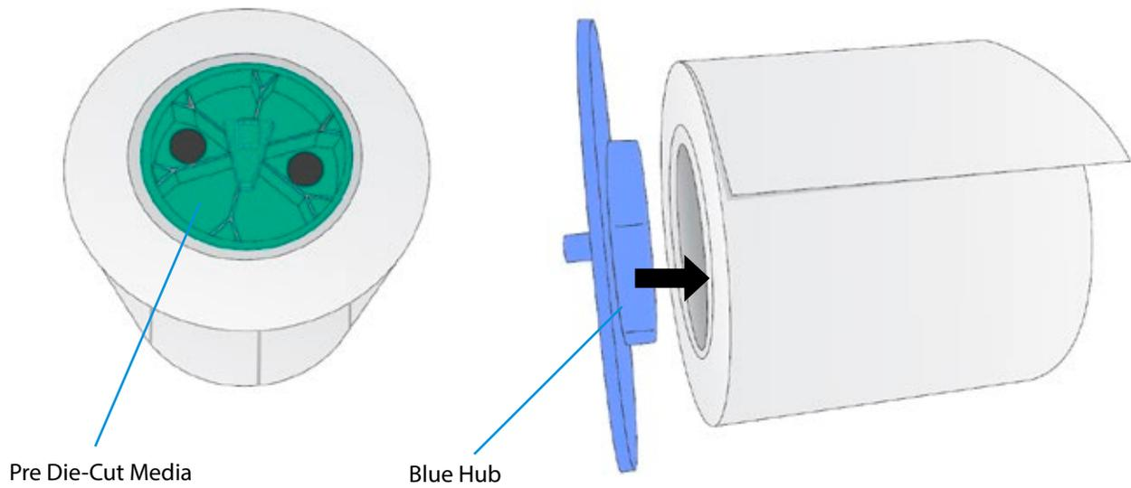
4. Set the roll in place so that the blue pin sits in the notch on the roll holder.
