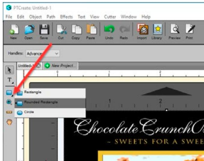
2. Before you start to draw the cut line, adjust the corner radius. You will not be able to change this after you draw your cut line. The corner radius is the amount of curve around the corners. .125 in (1/8 Inch) is the standard corner radius.
