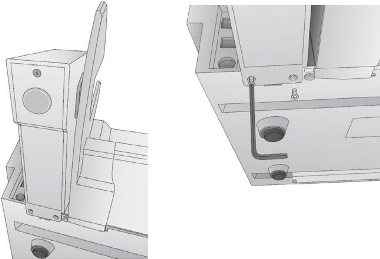
8. Install the T8 screws using the INCLUDED Allen key or a Torx T8 screwdriver.
