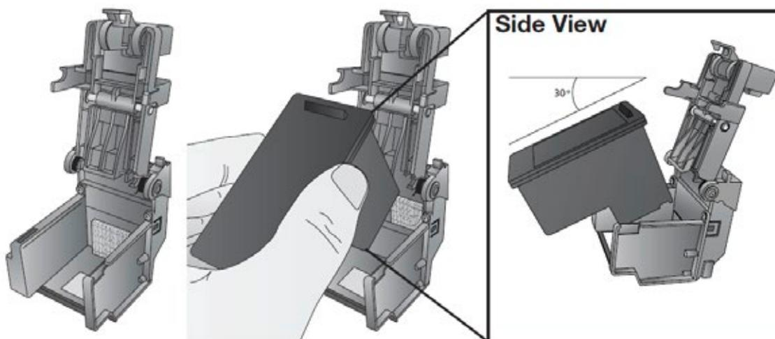
6. Make sure the cartridge is pushed back far enough so the ridge on the cartridge is behind the spring-loaded pusher on the lid. Push down on the cartridge. Close the lid on the cartridge by lightly pressing down from the top until you hear a click.
