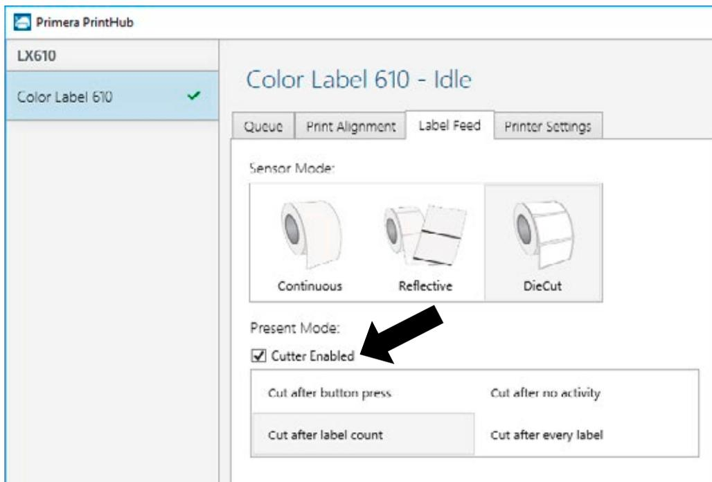
**Cut after button press.** This setting will cut after you press the Load/Feed button on the printer. This can be used after one label or an entire job. This feature is useful if you will not be present at the end of the print to catch the cut label.
