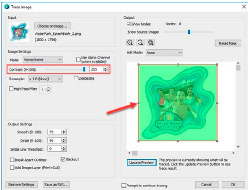
**Contrast to High:** If contrast is too high you will lose the shape detection and end up with a rectangle cut.
